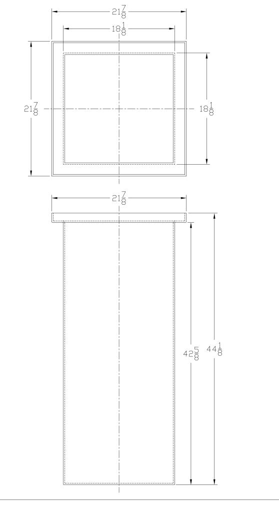
ALL DIMENSIONS SHOWN ARE OUTSIDE PART DIMENSIONS IN INCHES, AND VARY BY THE STANDARD ROTATIONAL MOLDING TOLERANCE OF  $\pm 2j - 3\%$ .
